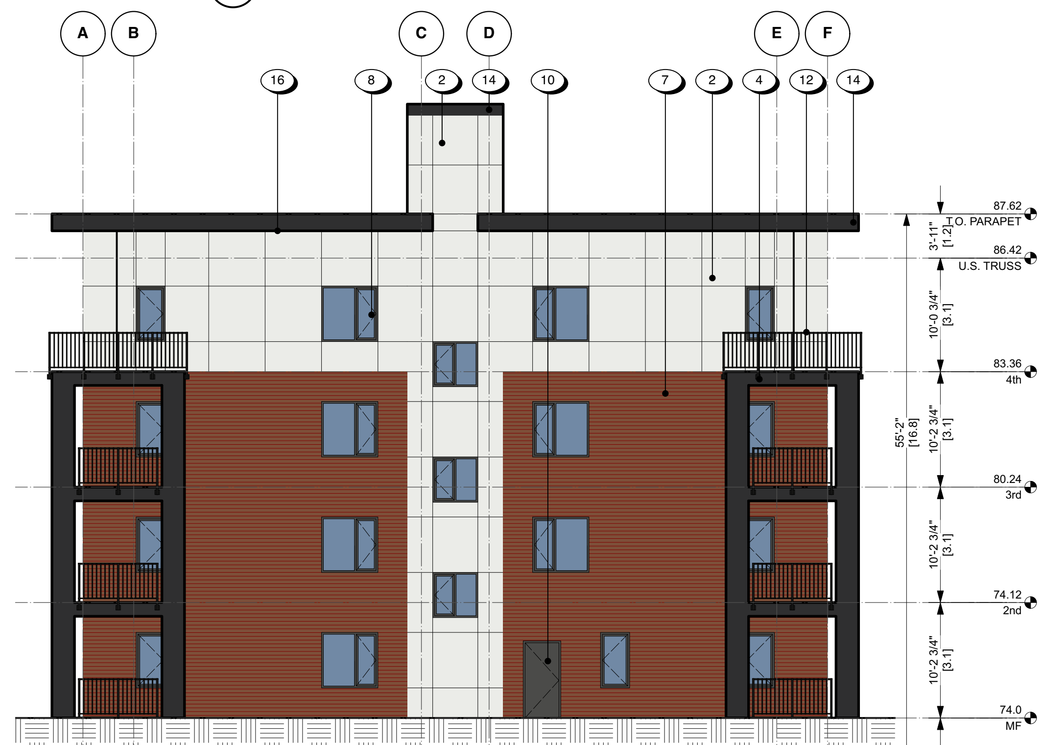
1 South Elevation - North Building A3.12 1:100
