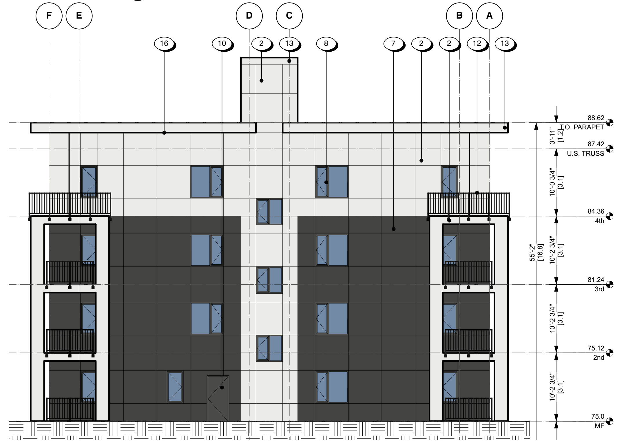
1 East Elevation - West Building A3.21 1:100
