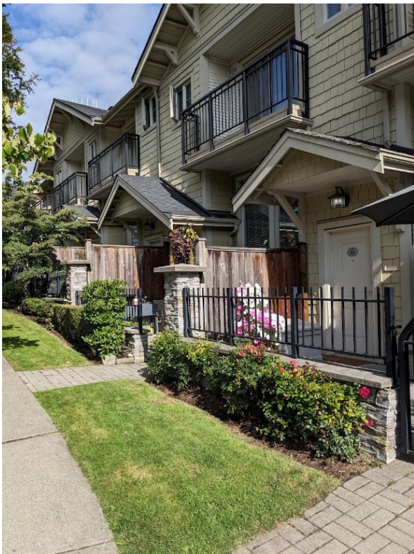
Figure 9: Private balconies and patios should use architectural techniques such as partitions/screens and step back to reduce visual and shadow impacts on neighbours (Guideline 42).
