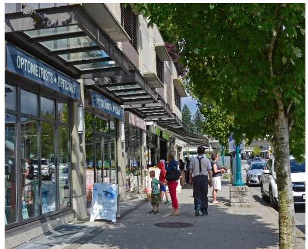
Figure 19: Prioritize pedestrian comfort through weather protective features such as canopies, awnings, and overhangs in locations such as primary building entrances, street corners, above store fronts and display windows, other areas where people frequently gather or wait. Ensure weather protection features are architecturally integrated and reflect the building's design and fenestration patterns (Guideline 49).
