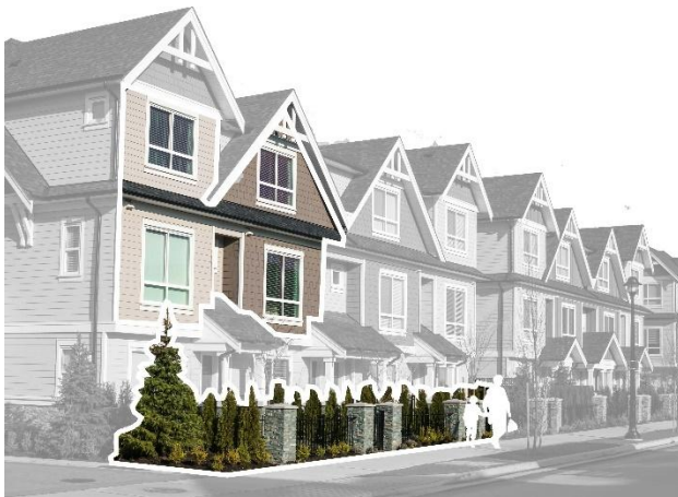
Figure 7: Fences should be of high-quality material and integrated with landscaping to minimize their visual appearance (Guideline 33).
