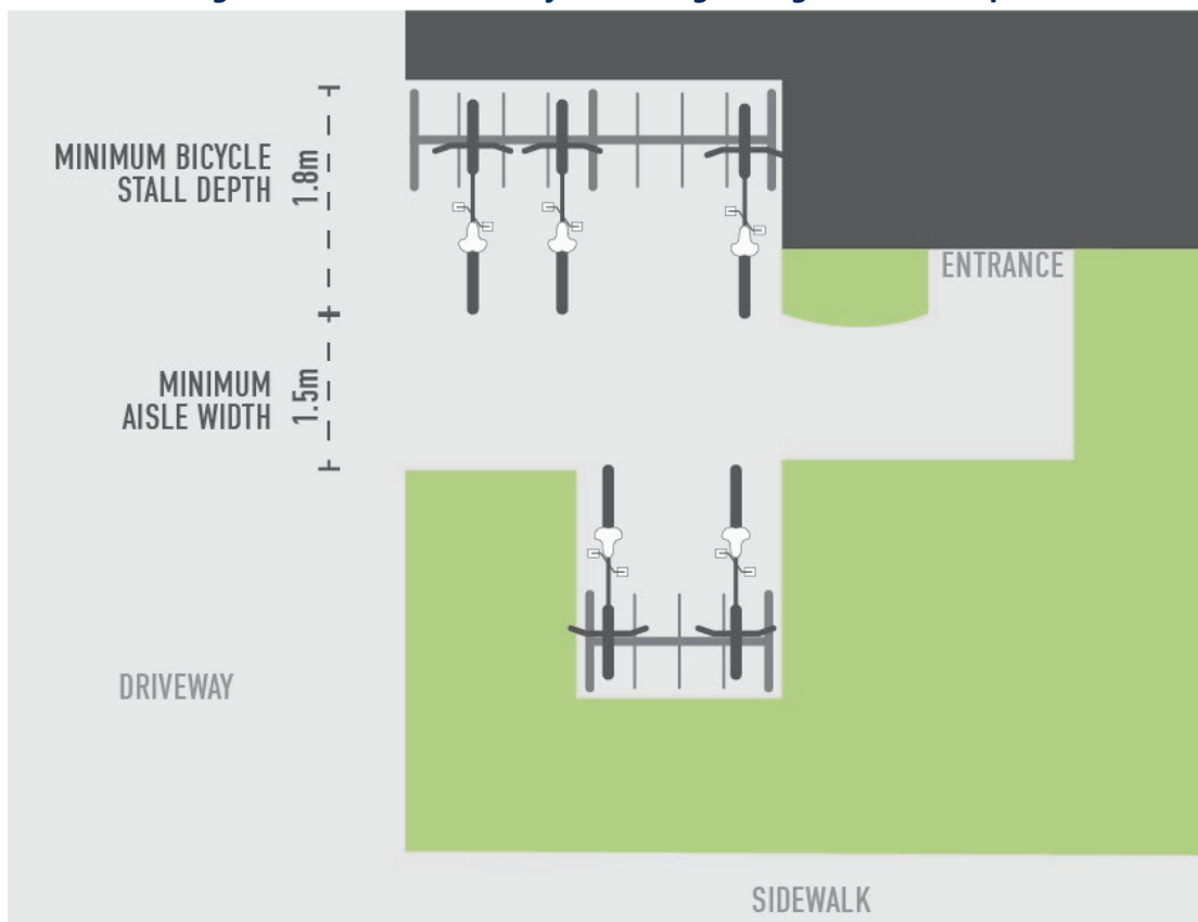
Figure 8-3. Short-Term Bicycle Parking Configuration Example
