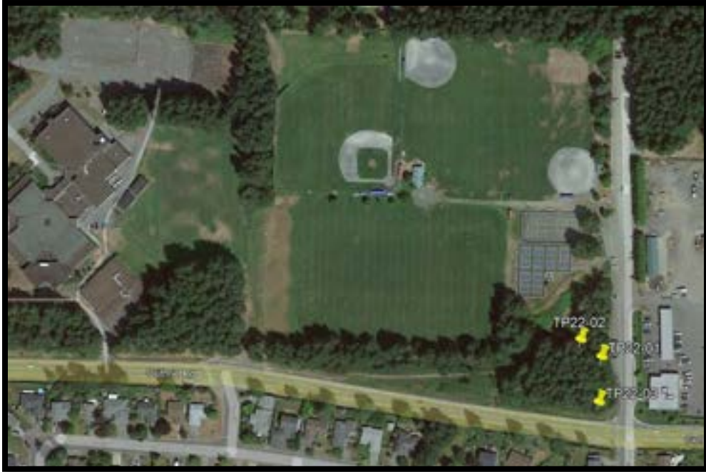
Figure 3- Approximate test pit locations indicated by yellow pins overlaid on Google Earth imagery of civic address 1519 Highridge Drive, Comox, BC. (Base image sourced from Google Earth, accessed on January 9, 2023).
