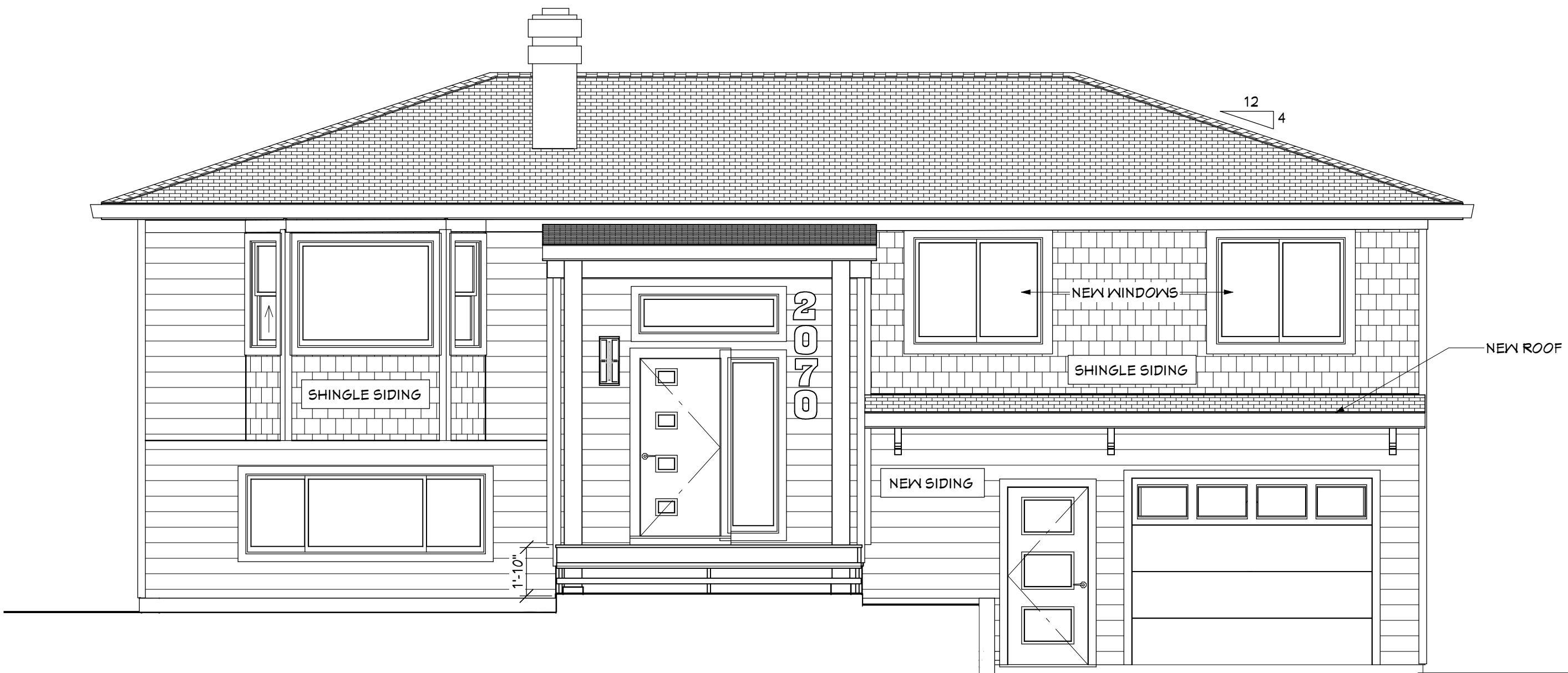
PROPOSED FRONT ELEVATION SCALE: 1/4" = 1'-0"
