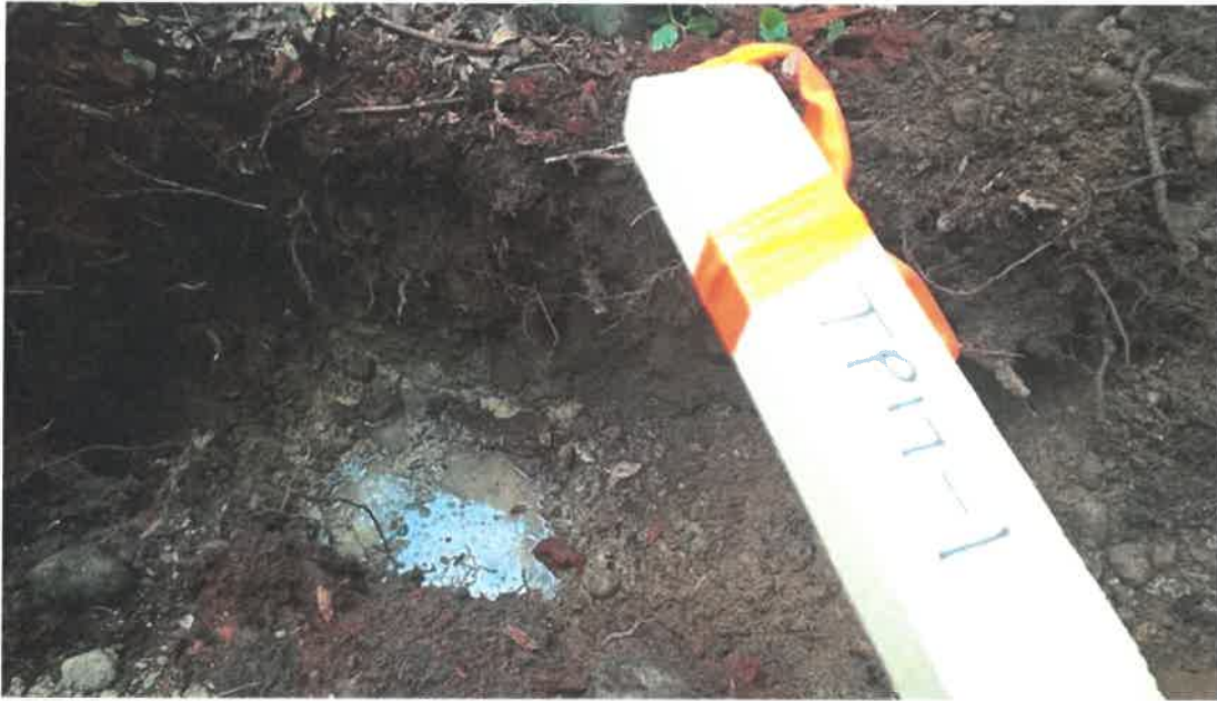
Photo 5 Test Pit TP17-01 shows typical shallow till and groundwater encountered approximately 0.7 m below ground surface.
