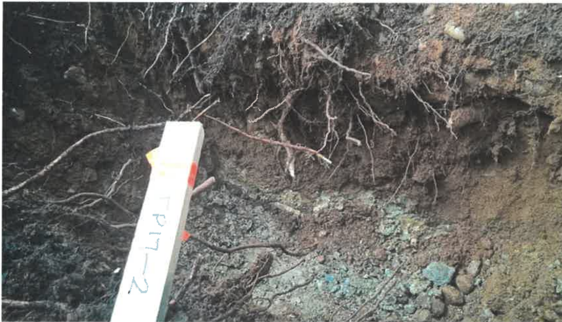
Photo 6 Test Pit TP17-02 shows typical shallow till and minor groundwater seepage approximately 0.8 m below ground surface.
