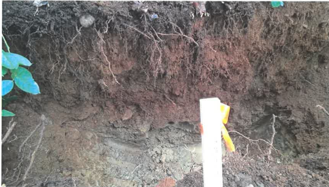
Photo 8 Test Pit TP17-7 shows shallow silty/clayey till and groundwater seepage approximately 0.9 m below ground surface.
