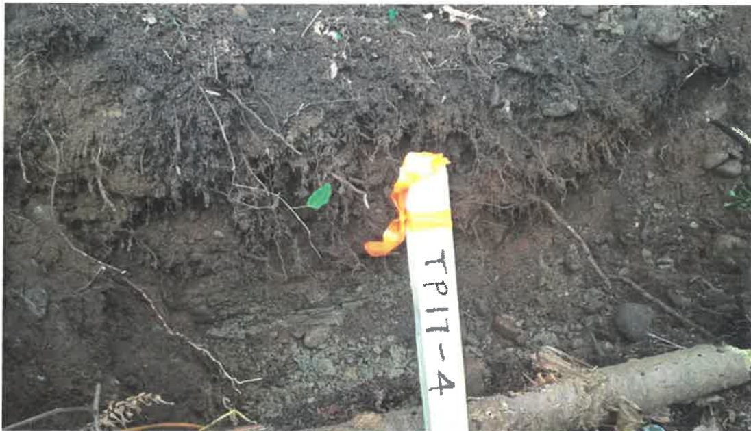
Photo 7 Test Pit TP17-4 shows typical organic material and brown fluvial sediments over shallow till.
