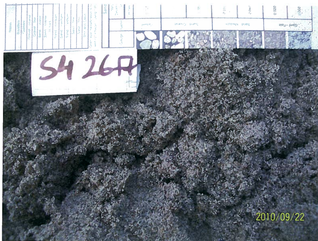
Photo 2: Clean sand of the Quadra Sands formation encountered in borehole S4 was deposited by glacio-fluvial meltwater. These sediments represent a great opportunity for infiltration of rain water.
