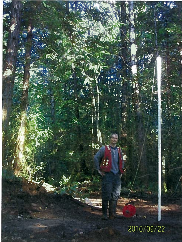
Photo 3: Measuring the water level in S6, in the northeast portion of the Site. Artesian conditions exist, with a water level 2.1 m above ground measured on September 23, 2010.
