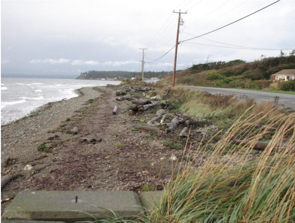
Photo 1: Viewing south, top of road el. = 3.8m, base of backshore el. 2.8m, WL = 1.0 m CGD (approximately).
